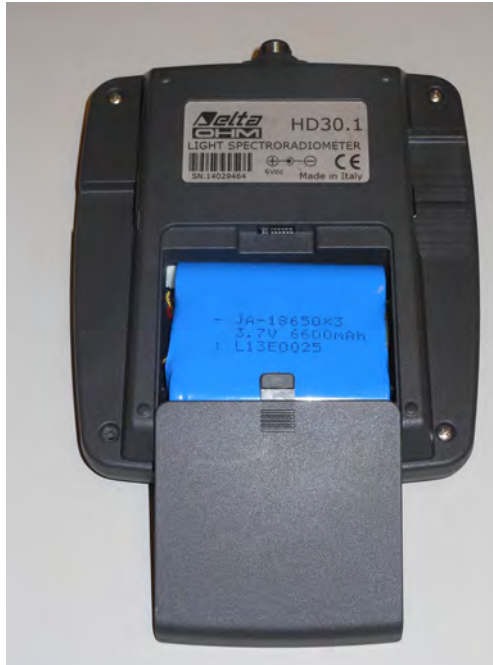
Figure 2.1: Disconnected battery inside battery compartment.
