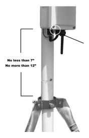
**Tripod Mount:** Ensure the distance between the bottom of the control box and the tripod is no less than 7 inches and no more than 12 inches.
