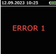
A screenshot of a mobile device screen. At the top, it shows the date and time '12.09.2023 10:25' and a battery icon. The main part of the screen is black with the text 'ERROR 1' in red. | <p><b>Error del sensor de presión</b></p> <ul style="list-style-type: none"><li>- El sensor de presión esta dañado.</li></ul> <p>Contacte al centro de servicio.</p> |
