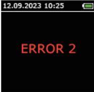
A screenshot of a mobile device screen. At the top, it shows the date and time '12.09.2023 10:25' and a battery icon. The main part of the screen is black with the text 'ERROR 2' in red. | <p><b>Error del sensor</b></p> <ul style="list-style-type: none"><li>- El sensor esta dañado.</li></ul> <p>Contacte al centro de servicio.</p>                       |
